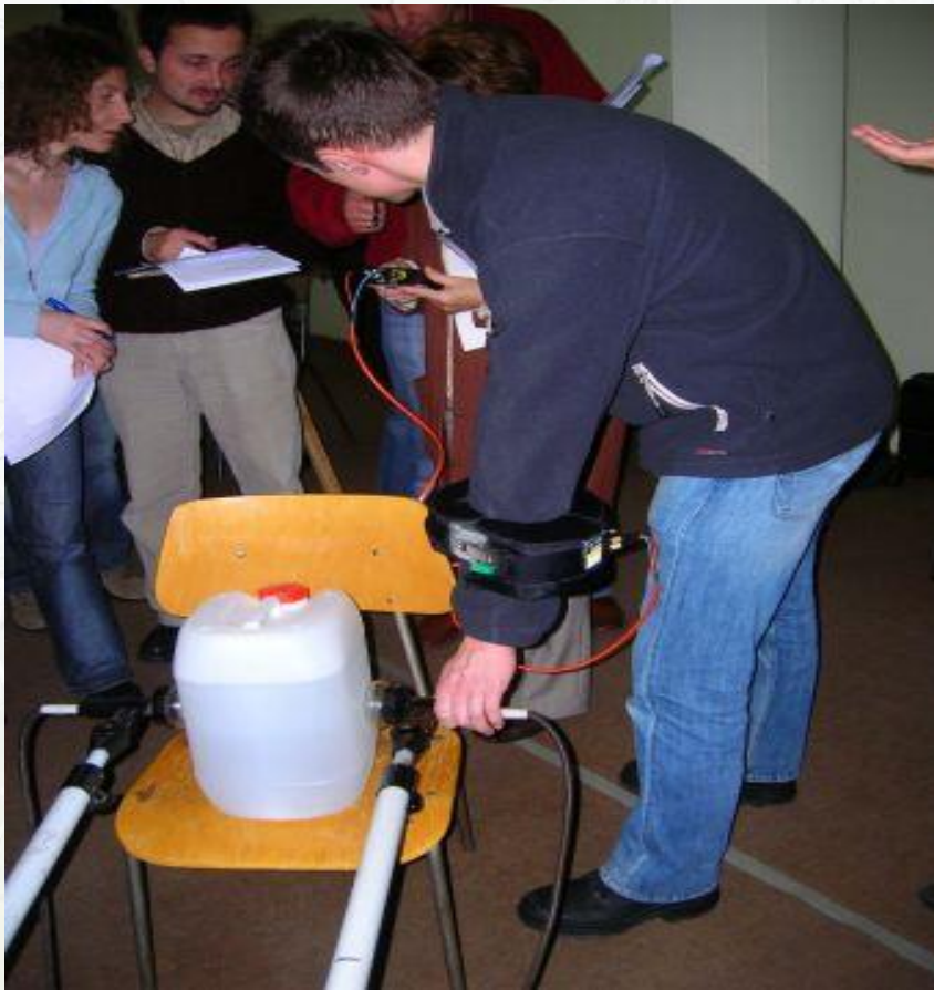
Fig. 2. Radiofrequency heat sealer and measurement of induced body currents.
