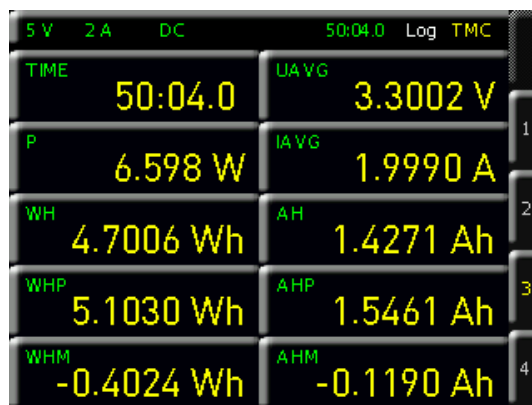
Fig. 6.23: Readout display with integrator output values.
