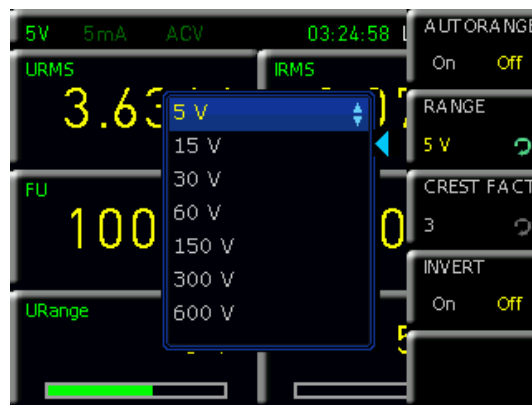
Fig. 5.8: Manual measurement range selection via ACQ menu
