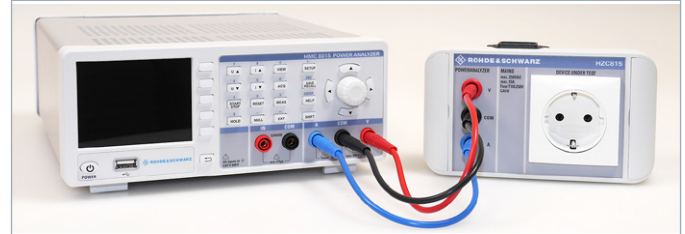
Fig. 4.1: Connecting HZC815 DE version to R&amp;S®HMC8015.
